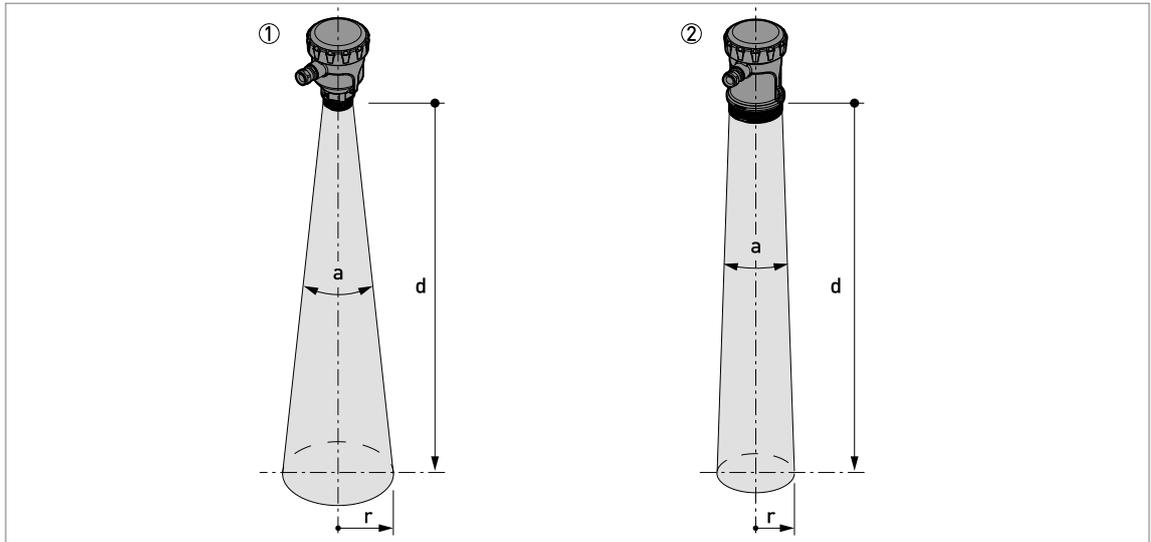
Figure 3-10: Beam angle
