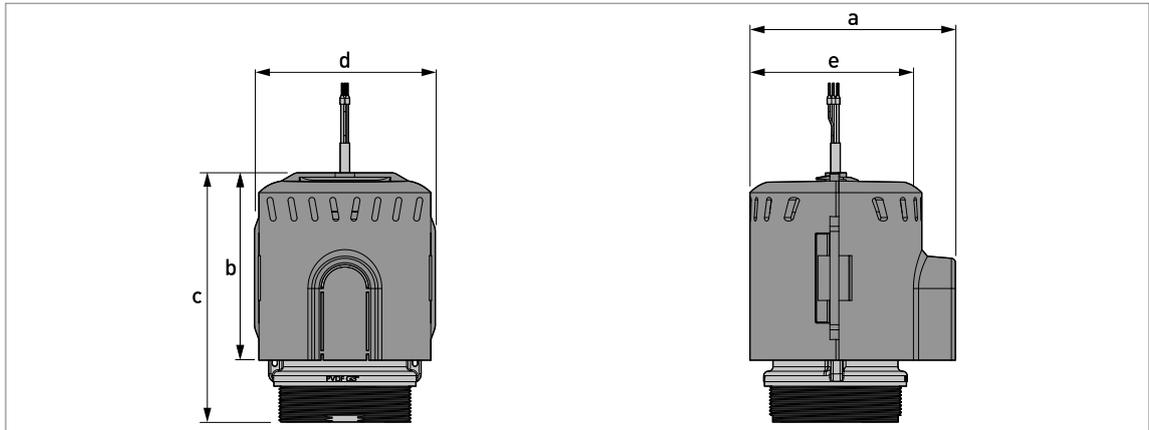
Figure 2-15: Weather protection cover attached to the OPTIWAVE 1530 / 1560
