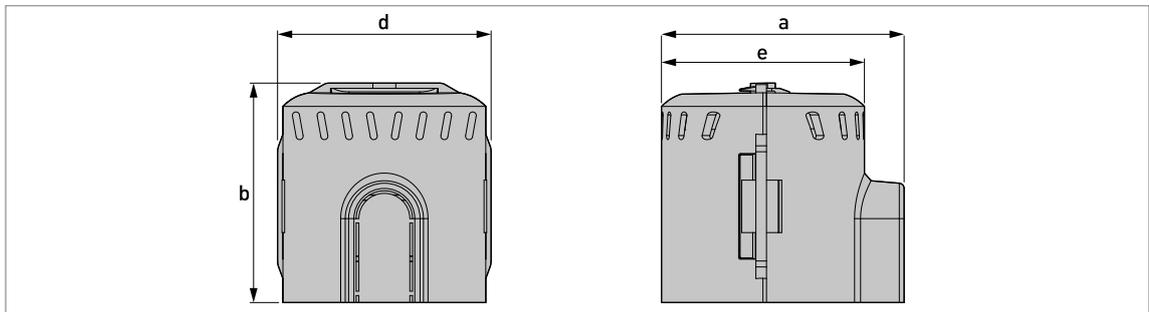
Figure 2-13: Weather protection cover (accessory)
