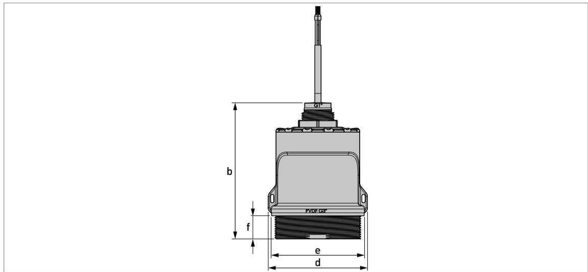
Figure 2-7: OPTIWAVE 1530 or 1560 with DN70 / 3" Lens antenna
