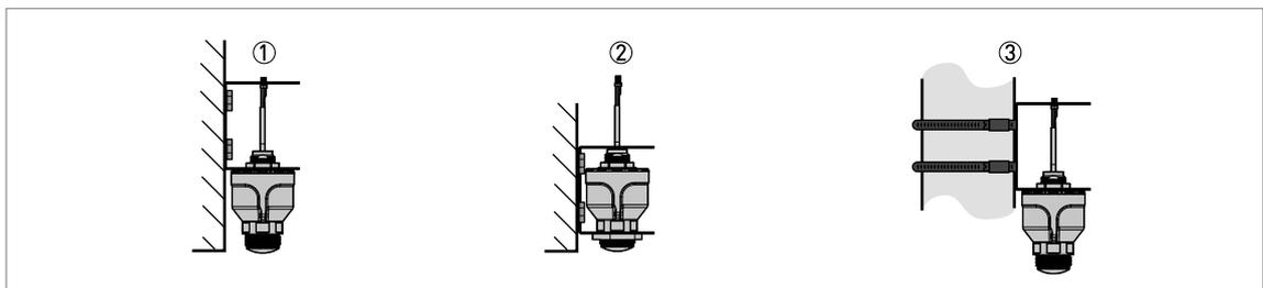
Figure 3-6: Installation on a wall or tube with a short bracket
