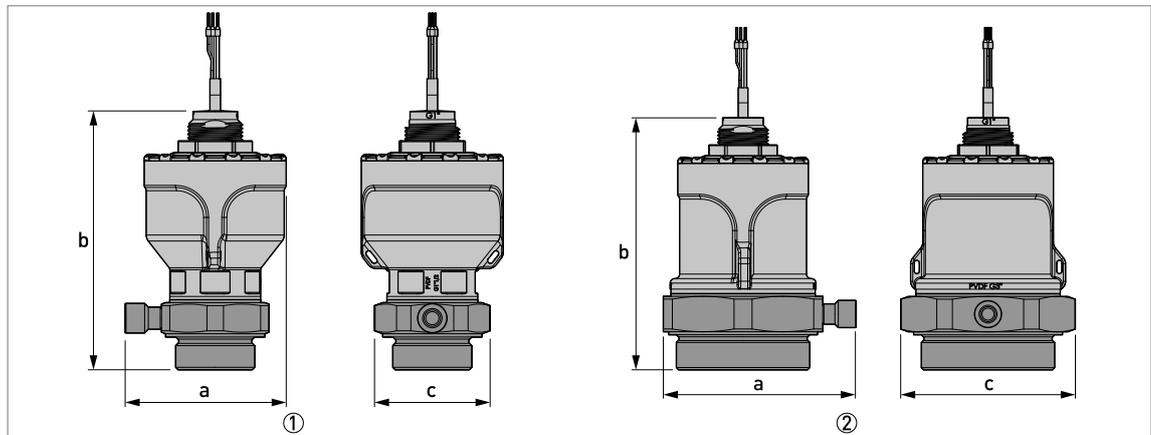
Figure 2-11: Purging system (accessory)
