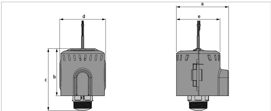
Figure 2-14: Weather protection cover attached to the device
