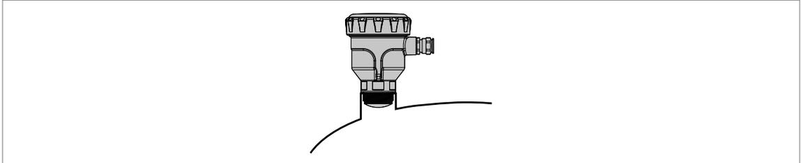
Figure 3-2: Threaded socket (NPT or G)
