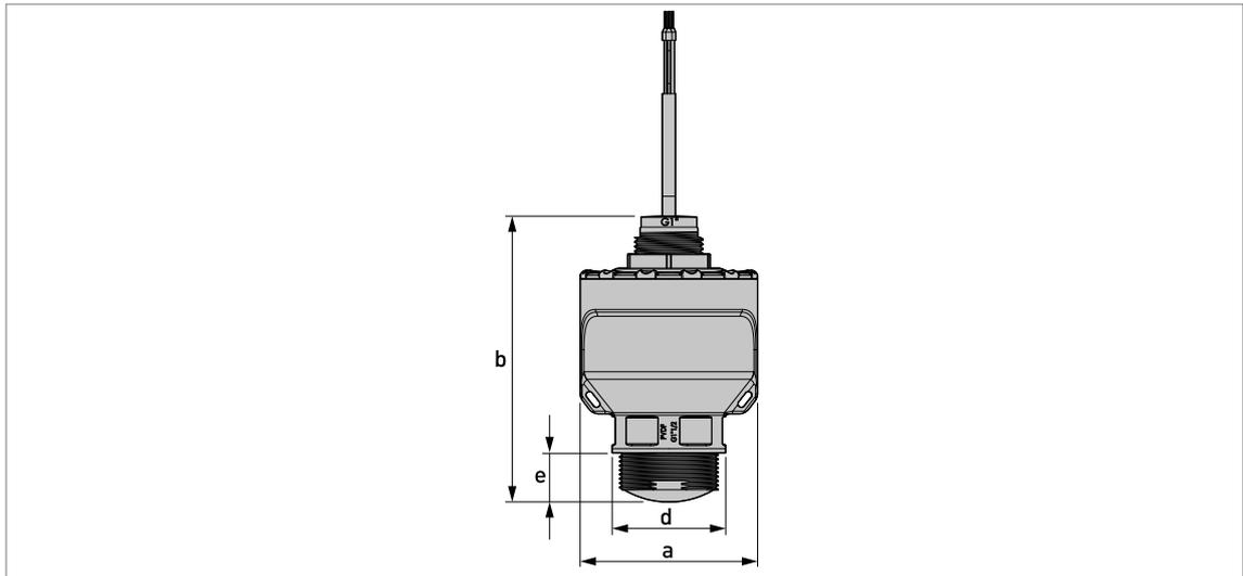
Figure 2-6: OPTIWAVE 1520 or 1540 with DN40 / 1½" Lens antenna
