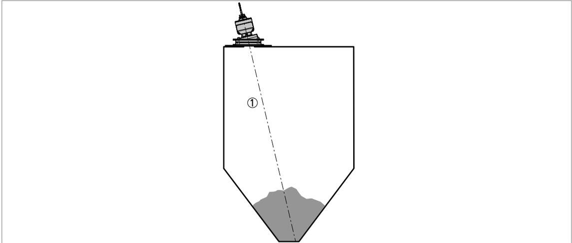
Figure 3-13: Tanks with dish-shaped or conical bottoms
